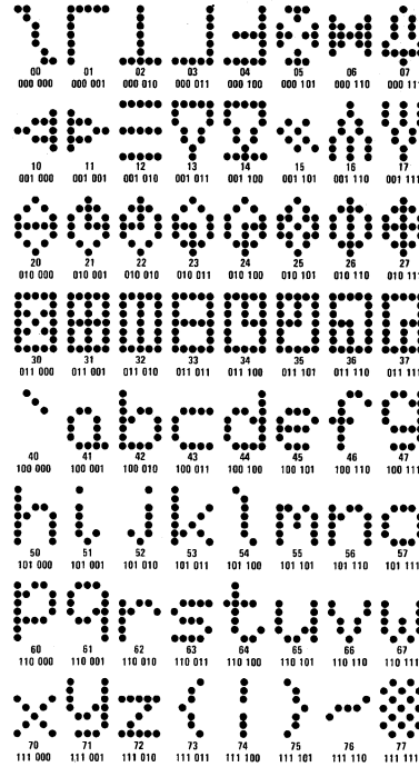
FIGURE 4. MM4240AE/MM5240AE Horizontal-Scan ASCII-7 Lower-Case Graphic and Control Symbol Subset
