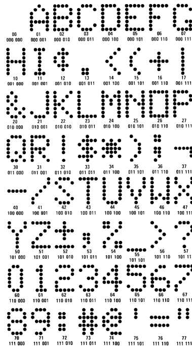
FIGURE 7. MM4240ACA/MM5240ACA Horizontal-Scan IBM EBCDIC Graphic Subset
