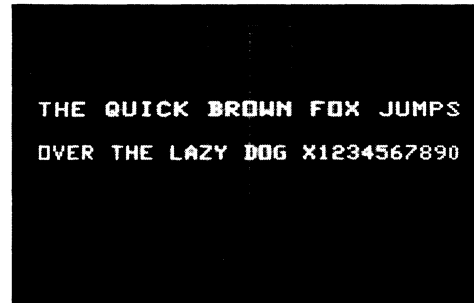
Figure 10b. Example of Character Generation Using Pedestal-type Scan.
